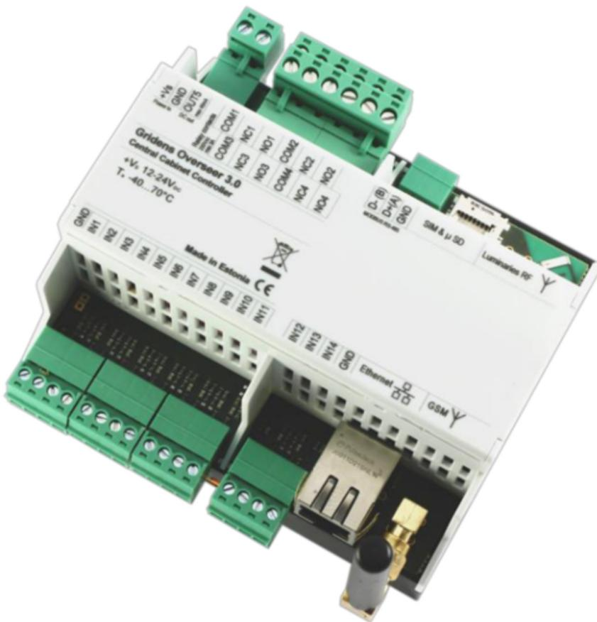
Main control unit and remote monitoring gateway.
